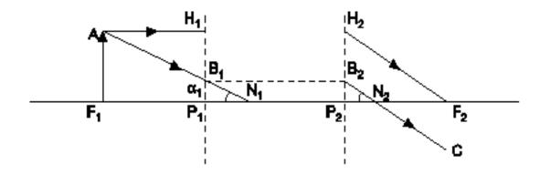
Consider a point in a first focal plane of an optical system. One ray  $AH_1$  is parallel to the axis. Its conjugate ray emerges along  $H_2F_2$  such that
