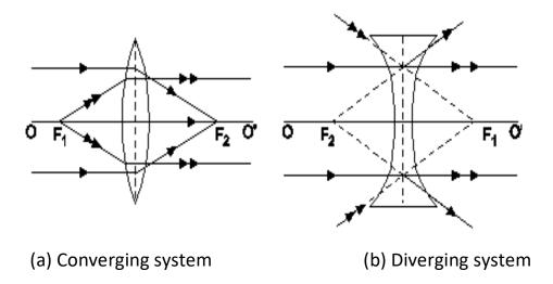
In a similar way, if the rays starting from (for a converging system) or directed towards (for a diverging system) an axial point F1, after refraction through the system become parallel to the axis OO' then such a point F1 is called first principal focus.
