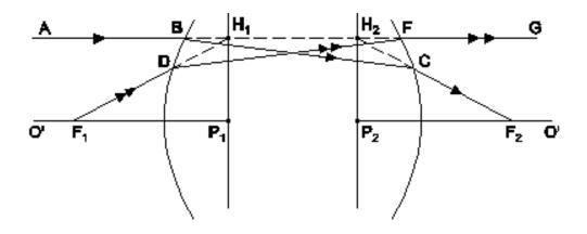
The plane passing through H2 and perpendicular to the principal axis OO' is termed as second principal plane of a lens. The point of intersection of this plane with the axis at P2 is called second principal point (P2).
